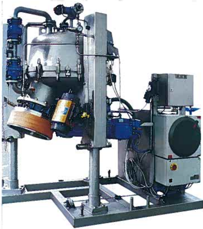
Pressure leaf filters are expensive and US biodiesel companies are reluctant to invest in today's economic climate
