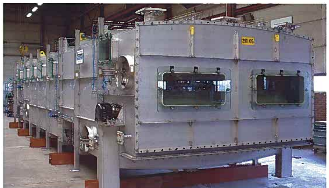
Horizontal vacuum belt filters offer multi-step processing on a single unit
